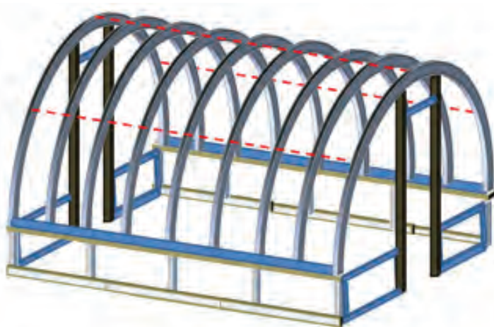
Figure 30. Red dashes indicate location of string lines for purlin locations.
