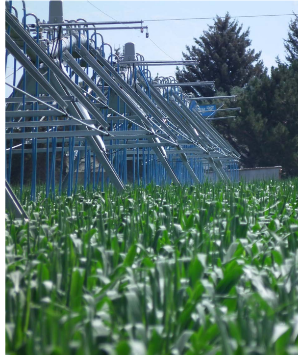
Linear move sprinkler in corn field.
