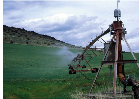
Top mounted sprinklers on a pivot can be less effective due to evaporation and wind affecting uniformity.
