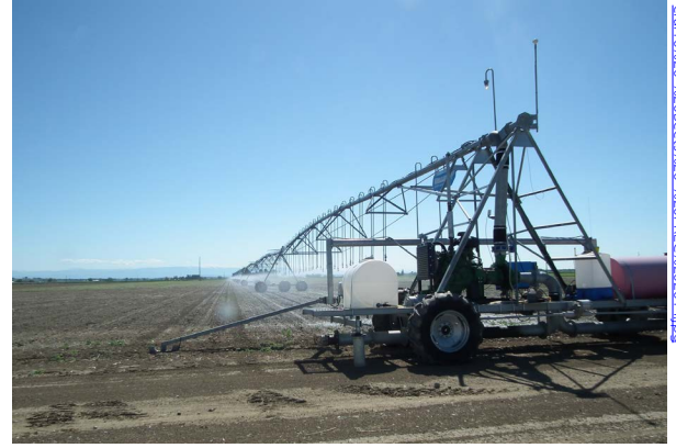
A diesel powered linear move sprinkler at the Powell Research and Extension Center, Powell, WY.
