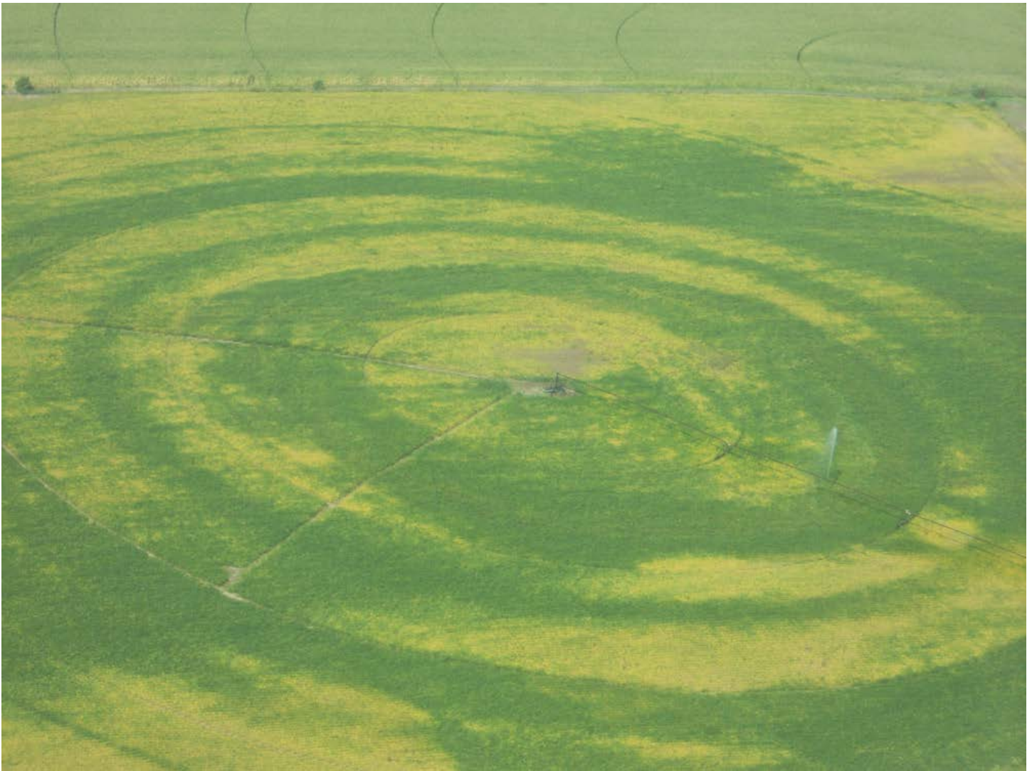
Figure 5. Aerial image of a center pivot irrigation system that has low application uniformity. (Courtesy UNL: Gary Zoubek)
