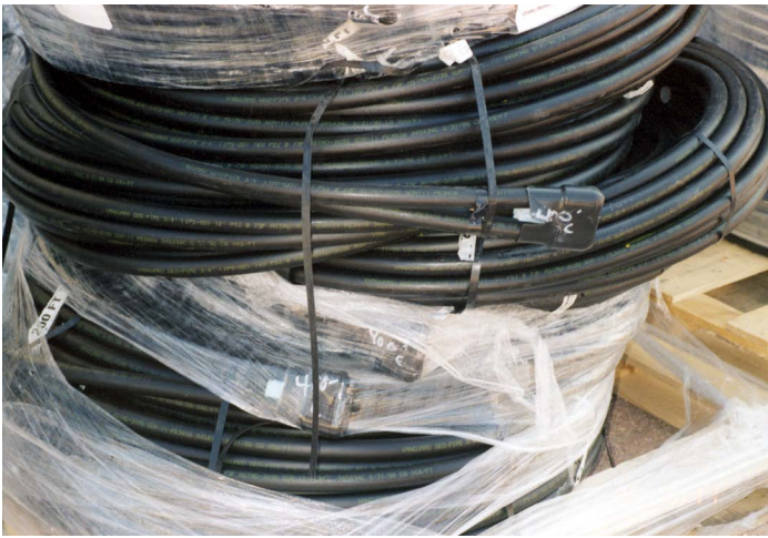
Polyethylene pipe Photo by John Barlean, NREL 07292 http://images.nrel.gov/viewphoto.php?imageld=6317366
