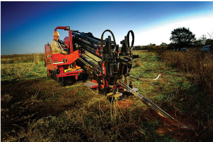
Directional drilling Photo by Ditch Witch. Licensed under CC 2.0 via Wikimedia Commons - https://commons.wikimedia.org/wiki/File:Ditchwitch_jt4020_mach1.jpg
