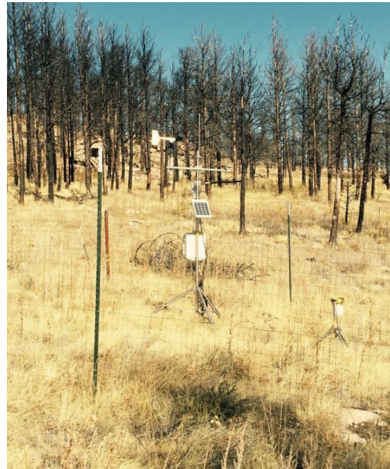
Figure 11. A weather station with remote access was installed at Rogers Research Site in 2013. That winter, however, mice climbed through a small opening in the bottom of the data logger box and caused extensive damage. UW irrigation specialist Vivek Sharma repaired the station in October 2017 (J. Tanaka, personal communication, 2017). It is recommended that standing dead trees in the vicinity of the station be removed to avoid further damage and, most importantly, to make the area safer for workers. (Photo by Linda van Diepen)
