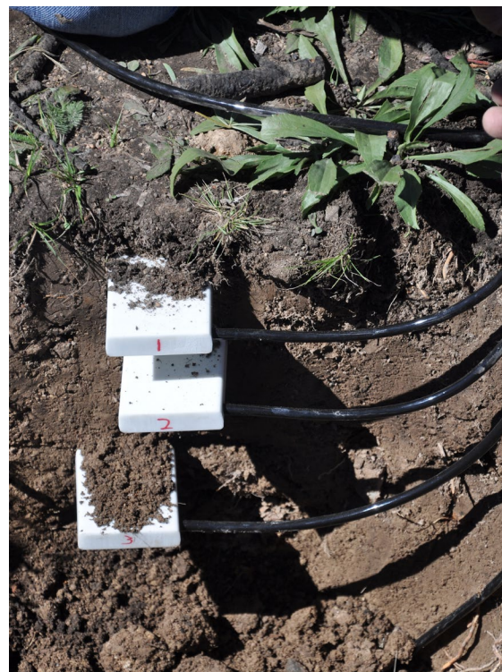
Figure 12. Soil moisture detection blocks were installed at the Rogers Research Site weather station to monitor soil water as part of the weather data set acquired for RRS. The blocks are set at 5, 10, and 20 cm (2, 4, and 8 inches) below the surface. Data, however, won't be acquired until repairs are made to the above-ground data logger, which was destroyed by mice shortly after being installed in 2013. This work is expected to take place in summer 2017. (Photo by S. Williams)
