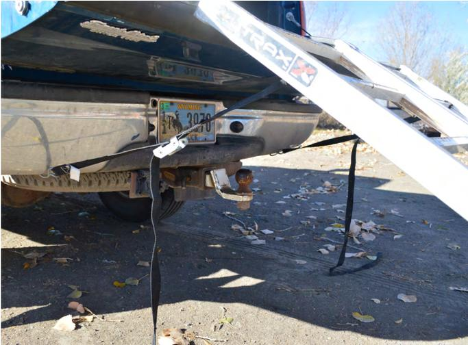
Ensure the trailer is still attached to the vehicle when loading and unloading. This might seem like common sense, however a trailer not attached to a vehicle can lift, move and slam to the ground which poses a risk to not only the rider, but also those around or near the trailer.
