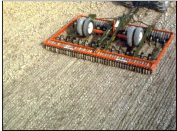
Cultipacking or roller-harrowing helps level soil, break up clods, push rocks into the soil surface, and firm soil for good seed-to-soil contact. (Photo credit: David Koch)
