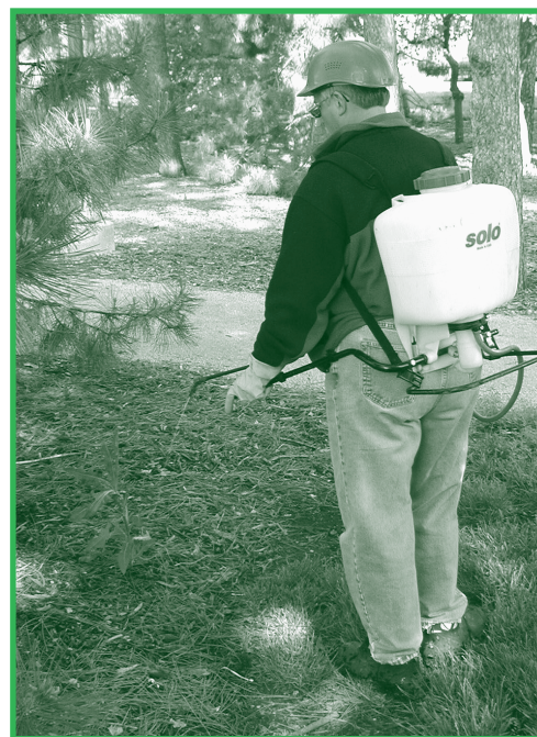
A backpack sprayer is a type of hydraulic sprayer.
