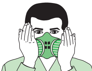
Positive pressure seal check
