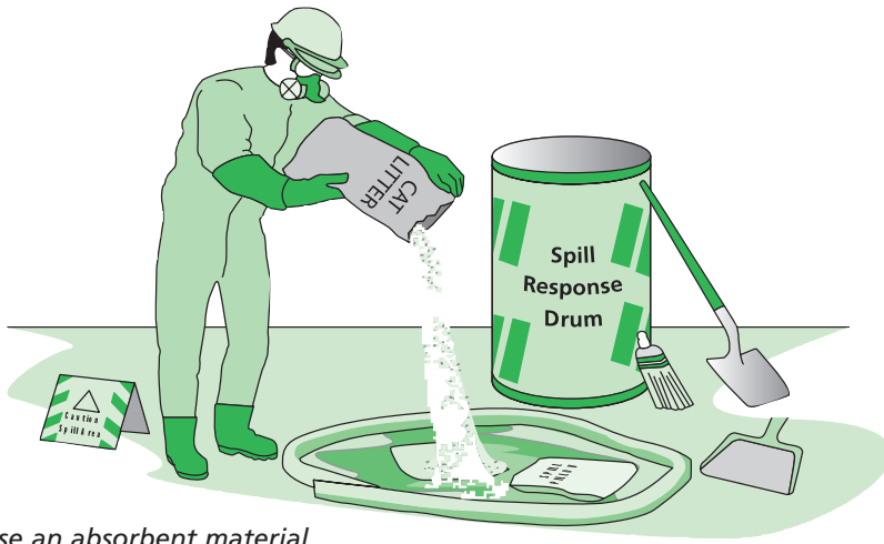
Use an absorbent material to help clean up a spill.
