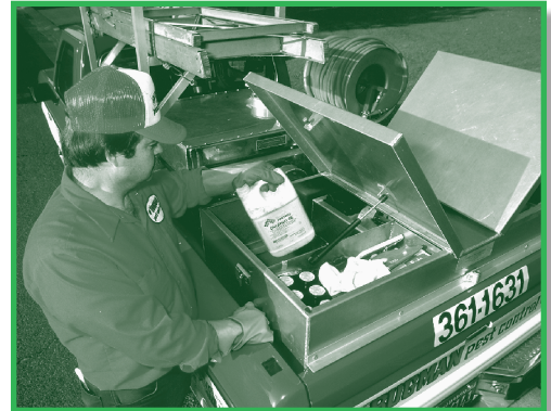
Cargo boxes allow for secure transport of pesticides and help prevent theft and vandalism.
