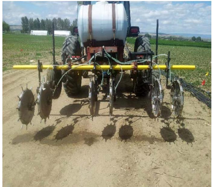
**Figure 4.** Liquid fertilizer applicators (above); side-dressing liquid nitrogen fertilizer at the Powell Research and Extension Center (below).
