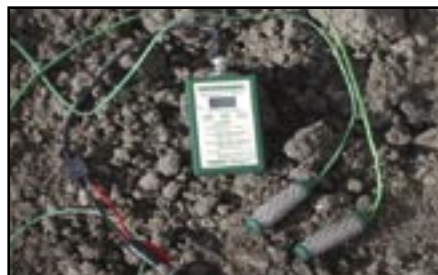
Place moisture blocks in at least two locations, at irrigation start and finish points and at 6", 18" and 30" depths.
