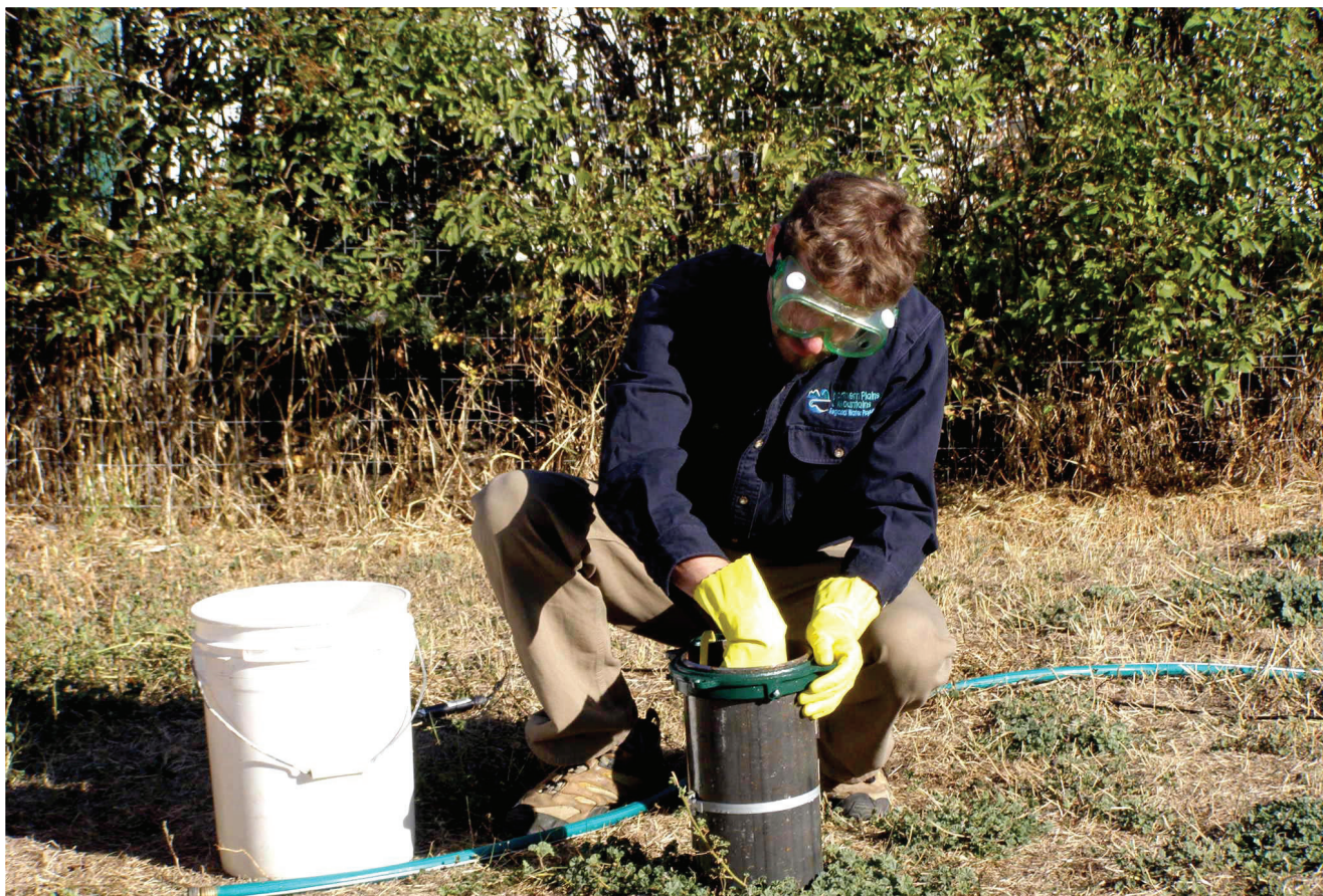
Adam Sigler (Montana State University) demonstrates the process of shock chlorinating a well for the “Taking Care of yOur Ground Water” DVD. Courtesy of Suzanna Carrithers Soileau, formerly Montana State University; currently USGS-Bozeman, Montana
