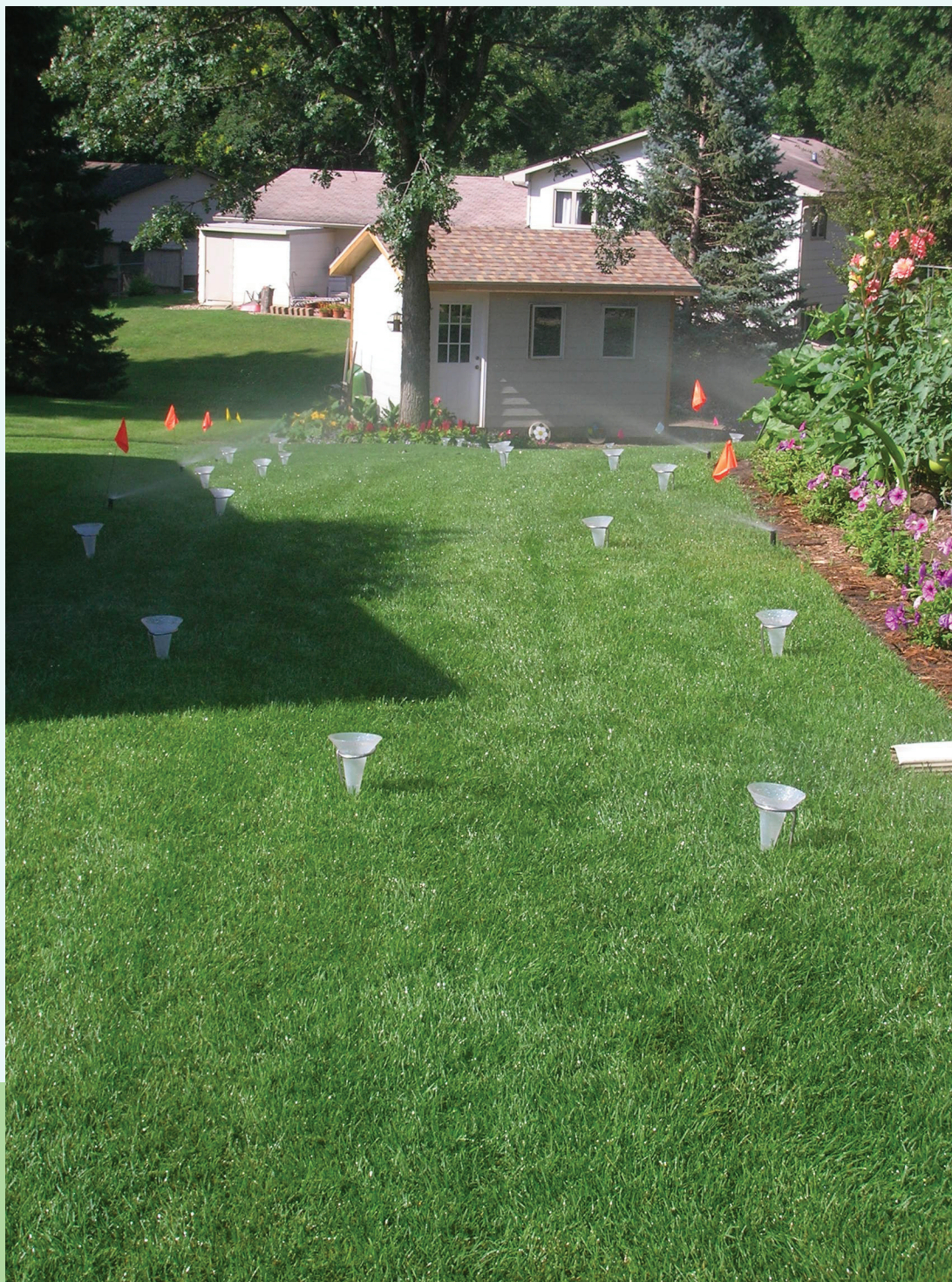
Irrigation uniformity measurement for residential irrigation sprinklers. Courtesy of Todd Trooien, Professor, South Dakota State University
