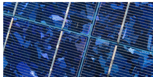
Close up of silicon crystalline solar cell. (Photo by Dennis Schroeder / NREL, 21770) Four, 250-watt PV panels = 1,000 watts = 1 kilowatt (kW). Together, they produce 1 kWh of electricity per hour in direct (peak) sun. If the panels get 4 hours of direct sun, the system may produce 4 kWh that day.
