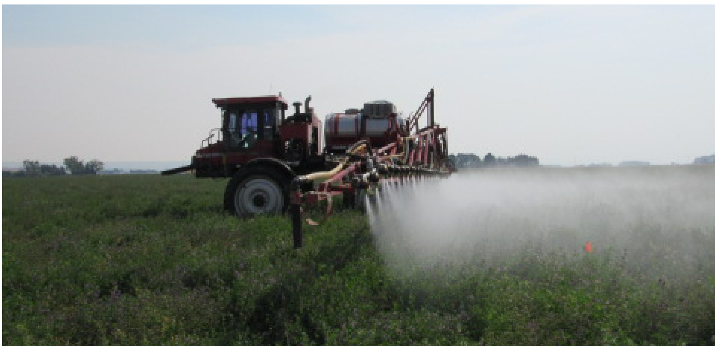
Figure 1. Case IH SPX 3300 applying desiccant to the test plots.
