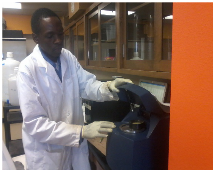
Figure 2. Hay baling at the Sheridan Research and Extension Center in June 2016 (left); forage nutritive value analysis using near infrared spectrophotometer at the University of Wyoming forage laboratory (right), December 2016.
