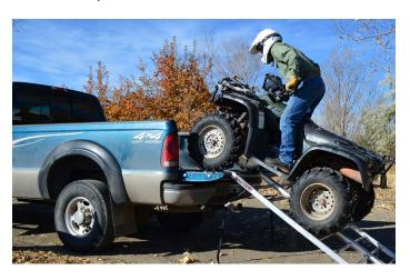
5 Maintain a low continuous speed for proper momentum while loading the ATV.
