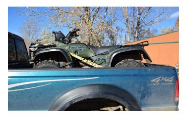
If not securing the ATV to a rigid surface, such as the bed of a pick-up truck, make sure heavy tie down straps are used to secure the front and back of the ATV. The suspension system of the ATV should be compressed at a minimum of several inches to ensure minimal movement during transportation. Frequent stops and checks is important when transporting ATVs, especially on trailers pulled over rough roads.
