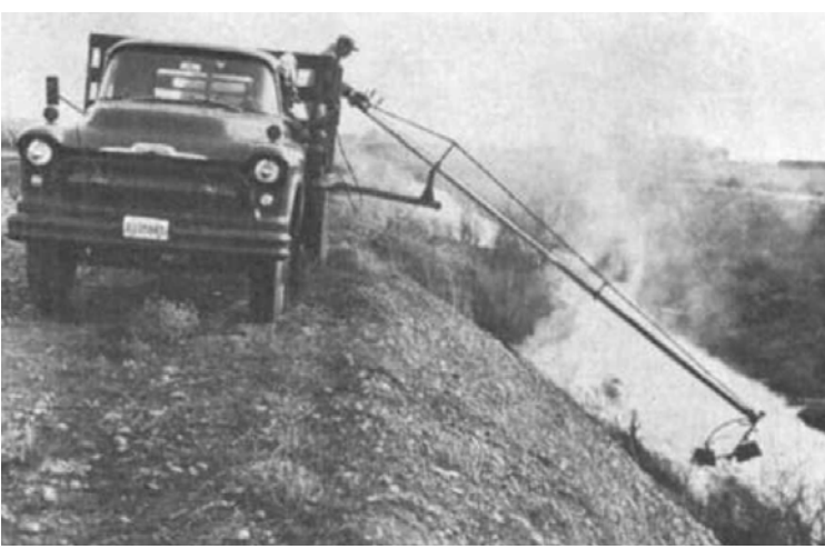
Figure 6. Propane gas burner with extended nozzle mounted on a truck [Image from Wallis et al. 1969. Burning weeds in drainage ditches to suppress population of green peach aphids and incidence of beet western yellows disease in sugar beets. Economic Entomology 62:307-309].
