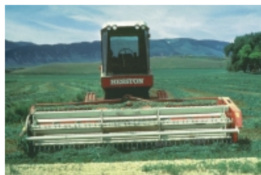
Figure 7. The accumulation of VW-infected leaves and stems on this swather header is a common way of spreading the VW fungus within and between alfalfa fields.
