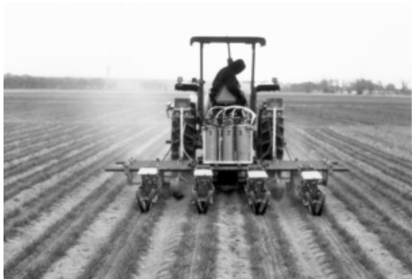
Photo 1. Herbicide application, herbicide incorporation and sugar beet planting operation in a cover crop.
