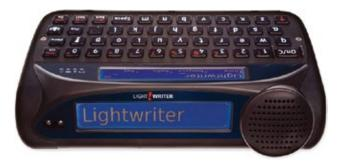
A portable text-to-speech device with dual displays, one facing the user and a second out-facing display, allowing natural face-to-face communication.
