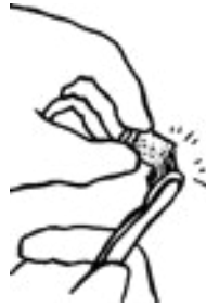
Use a brush to unclog nozzles
