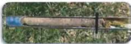
Figure 1. Soil sample core, discard portion to the right of the black line.
